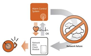
When the Network Alive Check Module detects an error, it quickly alerts the lone worker or other staff by means not dependent on the faulty system itself. It could be flashing lights or sirens. It can also reach any other designated personnel by SMS or through SCADA-systems.
