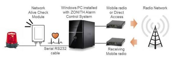
The Network Alive Check Module sends a "heart beat" to the Alarm Control System which transmits the heart beat onto the radio network. If there are no faults the heart beat is received by a receiving radio which passes it onto the Network Alive Check Module unit via the Alarm Control System. If the heart beat is not received by the unit it will go into alarm state.
